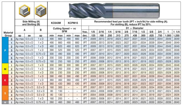
NOTE: Lower value of cutting speed is used for high stock removal applications or for higher hardness (machinability) within group.
