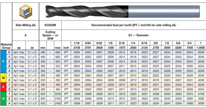
NOTE: Lower value of cutting speed is used for high stock removal applications or for higher hardness (machinability) within group.
