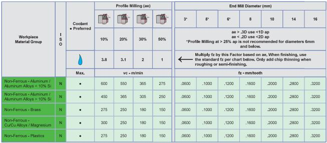
Above 20,000 RPM, Tool Balancing Required
